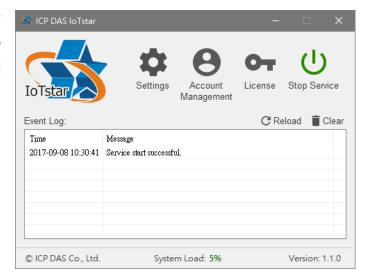
"License" the setting window, it will display the Information as "Registration status", "Maximum number controllers of can be connected with IoTstar" and "function status of the optional package".
